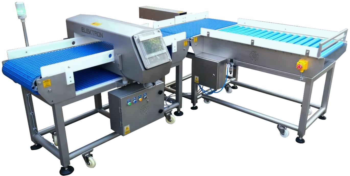
Metal detector with roller deflector for E1 and E2 boxes and for cardboard boxes.
