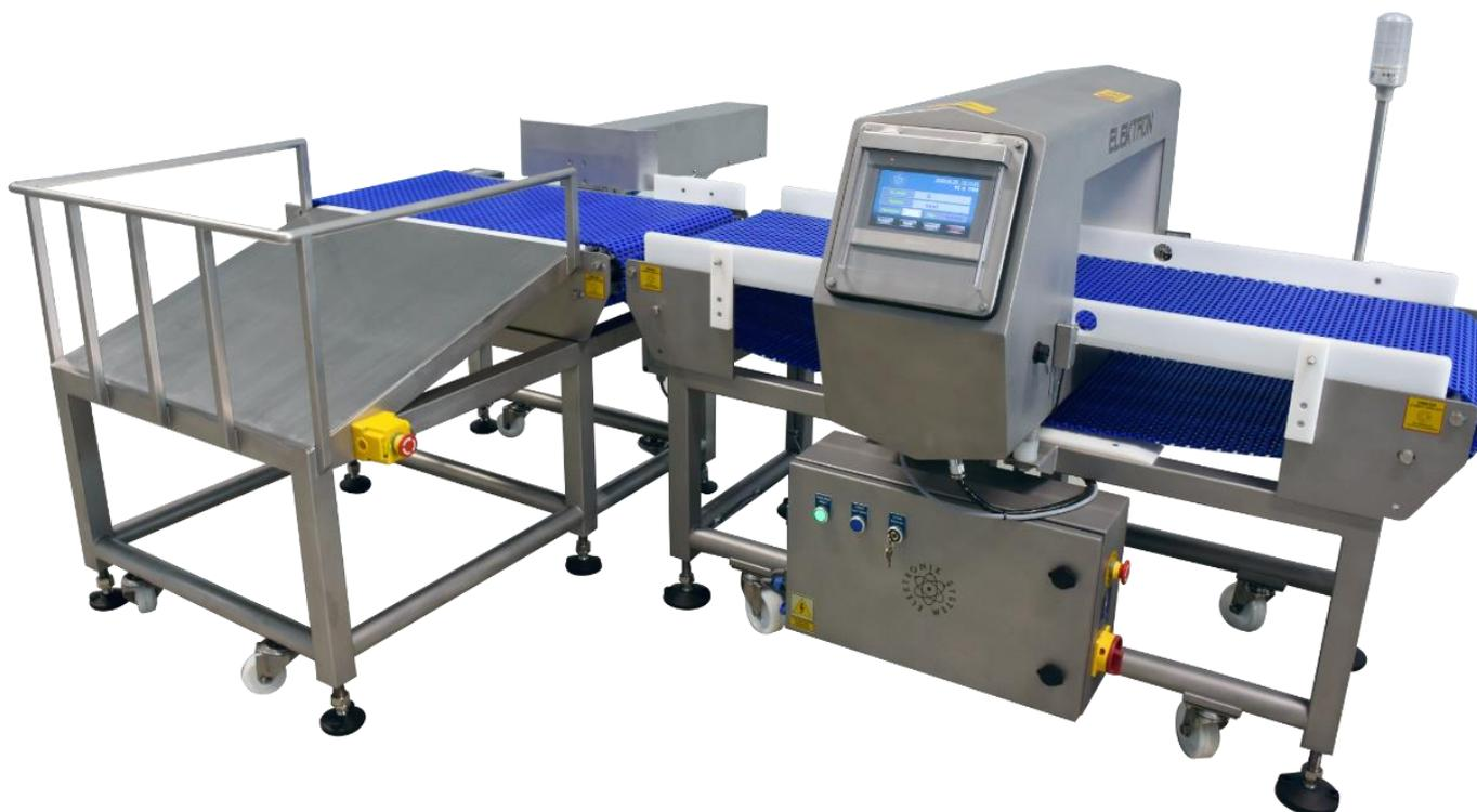
Metal detector with a ramp for products packed in bags or cartons.
