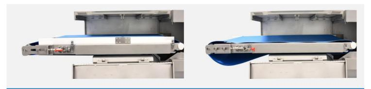
After dismantling the side guide, simply release the tensioning element and the tape is ready to be removed.
