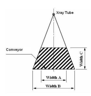
Type and type of X-Ray scanner we select according to the requirements client. The product dimension must be inscribed in the detection cone accordingly with table.
