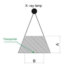
The type and type of the X-Ray scanner are selected according to the customer's requirements. The product dimension must be entered in the detection cone according to the table below.
