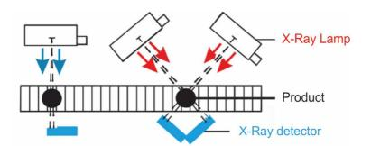
The technology of combining three beams that examine the product, provides the highest level of detection.
