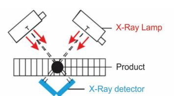
The technological connection of two beams examining the product ensures a high level of detection.
