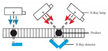
Three-beam connection technology researching the product, provides the highest detection level.
