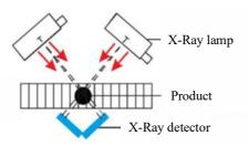
Technological connection of two beams researching the product ensures high detection level.
