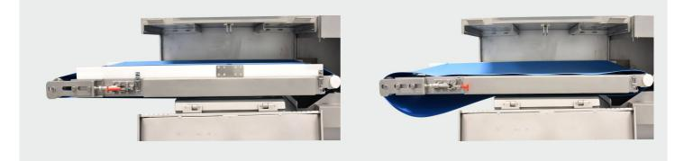
After removing the side guide, all you have to do is release the tensioning element and the tape is ready to be removed.
