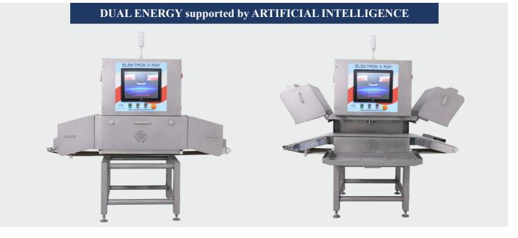
This X-Ray scanner has the highest detection level among X-Ray scanners, especially for the elimination of bones and bones as well as other foreign bodies such as glass, rubber, plastic. This is due to the latest technology **DUAL ENERGY**.
