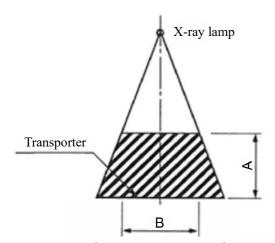
We select the type and type of X-Ray scanner accordingly with customer requirements. Product dimension must be inscribed in the detection cone according to the table below.
