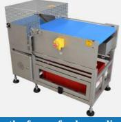
A trapdoor in the form of a descending transporter Reject system designed for long products with a closed area and a lockable container.
